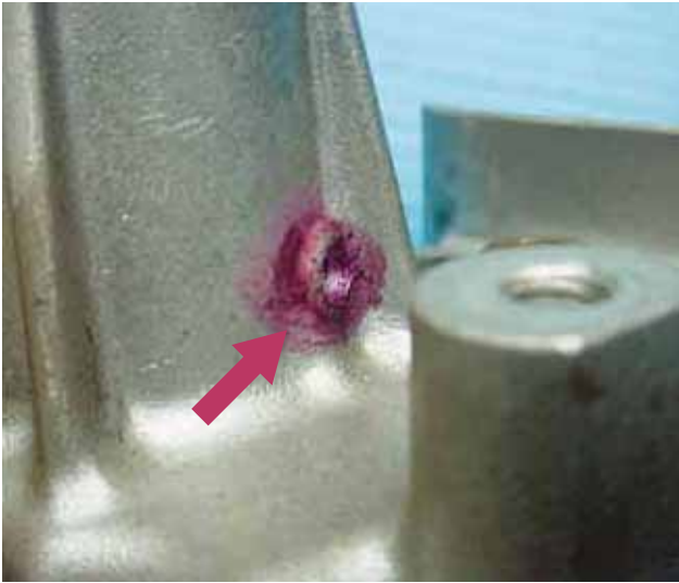
Normal Dried coolant residue.
