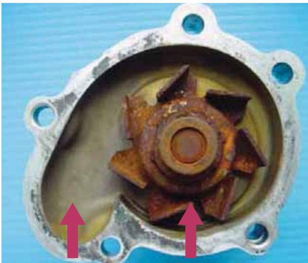
Contamination of water pump body
