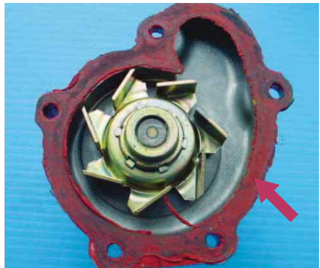
Gasket performance has degraded.
