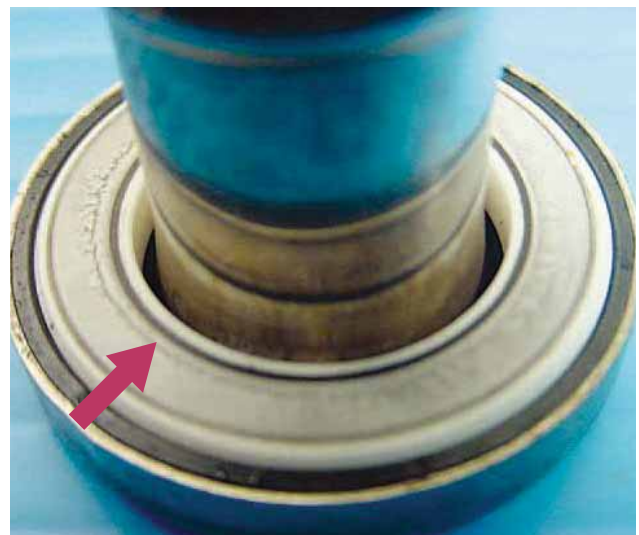
Damaged Accumulated sludge (Contaminated coolant).
