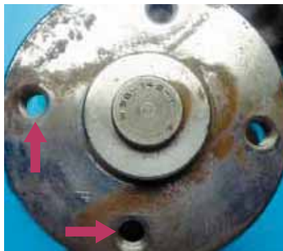
Damage at the stud bolt ends
