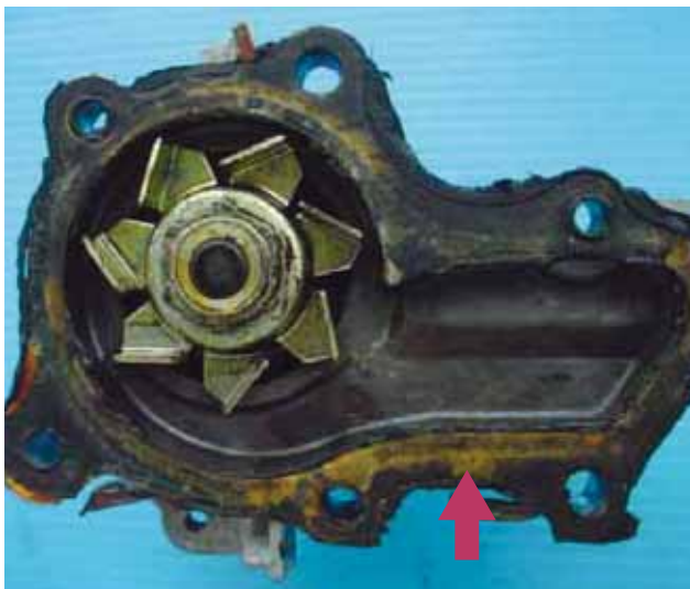
Insufficient accuracy on the mounting surface.
