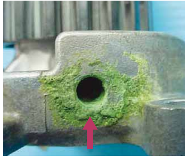
Damaged Large coolant bleed mark, dampness or dripping.
