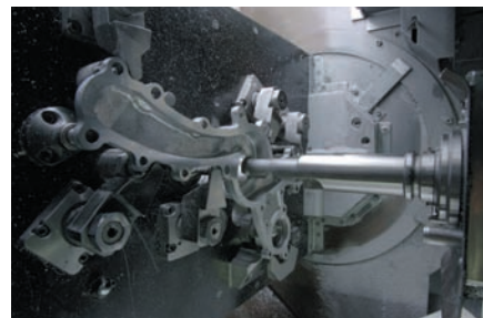
High precision machining process for Water Pumps
